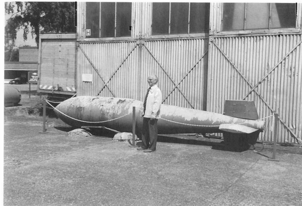
A Tallboy bomb on display at the Brooklands Museum near Weybridge in Surrey. These enormous devices, with precision machined cases made from especially hard steel, were the first to cause serious damage to U-boat bunkers and some of them even pierced through seven metres of reinforced concrete.
